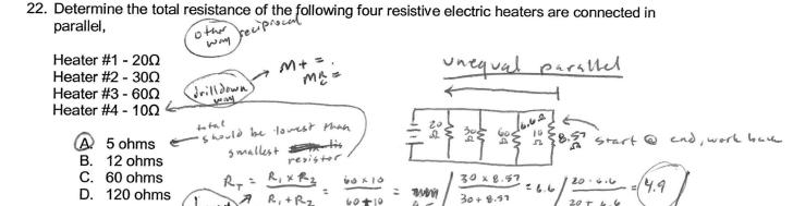
23. If the above parallel circuit was supplied by a 240volt, single phase, power source, what would be the total current?
